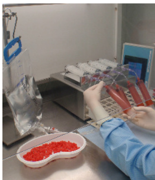
Fig.1: Filling with a four-channel-syringe pump
