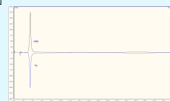
Figure 1 and Table 1: Only one peak in SEC was found. The retention time and AUC did not change after 6 months at 4°C.
