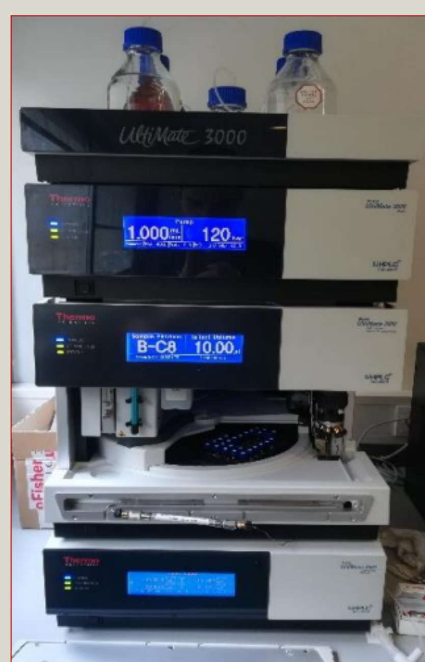
Image 1. UltiMate 3000 HPLC (Thermo Fisher Scientific, USA): stability tests Image 2. Mastersizer 300 (Malvern Panalytical, UK): particle sizes tests
