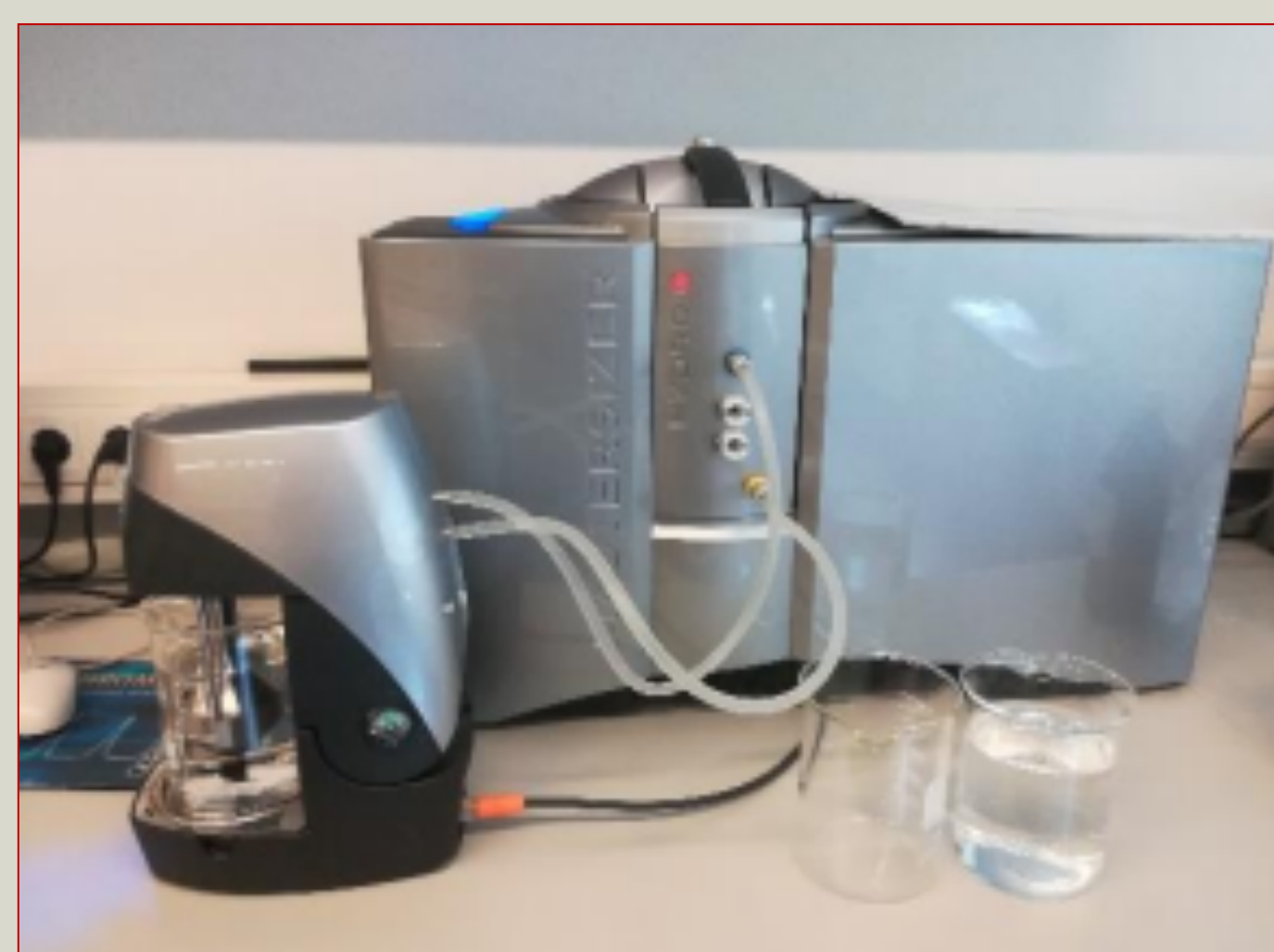
Image 1. UltiMate 3000 HPLC (Thermo Fisher Scientific, USA): stability tests Image 2. Mastersizer 300 (Malvern Panalytical, UK): particle sizes tests
