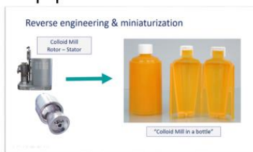
Figure 1: Enclosed wet milling device that produces uniform particles leading to palatable high-quality liquid formulas with the required dose uniformity
