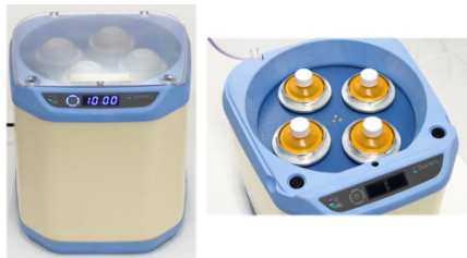
Figure 2: Milling unit closed and opened showing containers in place
