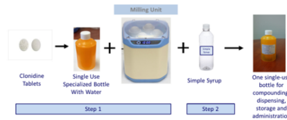
Figure 4: Compounding process for oral liquids using specialized plastic containers
