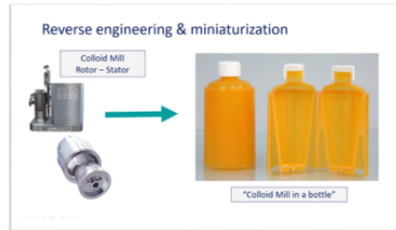
Figure 1: Enclosed wet milling device that produces uniform particles leading to palatable high-quality liquid formulas with the required dose uniformity
