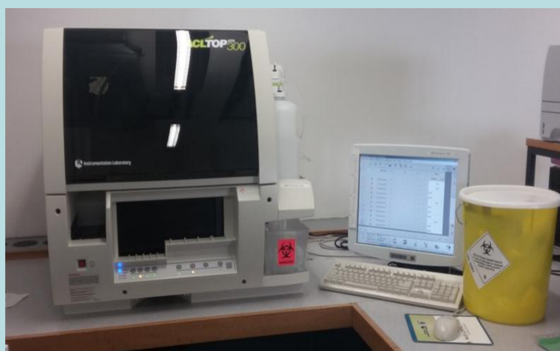
Fig. 2. The ACL TOP 300 robot for used for the heparin assay, Assay of Heparin Ph. Eur. 2.7.5..
