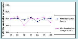
Graph 3: Evolution of concentrations of 25 mg/mL azacitidine suspensions after freezing at -20°C
