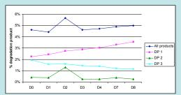
Graph 4: Evolution of degradation products (DP) after freezing, defrosting and storage for 8 hours at 2-8°C
