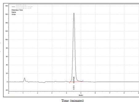
Chromatogram of sodium thiosulfate 180 µg/mL in NaCl 0.9% without stressed conditions.
